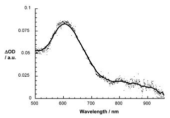
*Figure 8.* Picosecond transient absorption spectrum (visible–near-infrared part) recorded with a 100 ps upon flash photolysis of dyad **Co3** ( $\sim$ 5.0 × 10<sup>-5</sup> M) at 532 nm in deoxygenated benzonitrile, indicating the Co(II)P  $\pi$ -radical cation features ( $\lambda_{max} = 600$  nm) – Co(II)P<sup>++</sup>.
