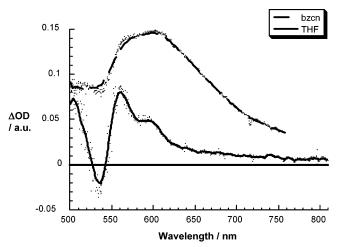
*Figure 12.* Picosecond transient absorption spectrum (visible part) recorded with a 100 ps upon flash photolysis of dyad Co1 ( $3.0 \times 10^{-5}$  M) at 532 nm in deoxygenated THF (solid line) and benzonitrile (dashed line).
