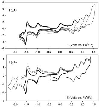
**Figure 4.** Cyclic voltammetry (v = 0.1 V/s) of **Co1** in benzonitrile and 0.1 M Bu<sub>4</sub>NPF<sub>6</sub> for different anodic (top) or cathodic (bottom) switching potentials.
