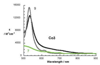
**Figure 2.** Absorption spectra of CoTt-BuPP (9), Co3, and  $trans-2-C_{62}$ -(COOEt)<sub>4</sub> (7) in toluene.
