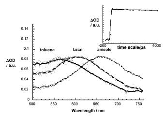
**Figure 10.** Picosecond transient absorption spectrum (visible part) recorded with a 100 ps upon flash photolysis of dyad **Co3** ( $\sim$ 5.0 × 10<sup>-5</sup> M) at 532 nm in deoxygenated toluene ( $\lambda_{max} = 565$  nm), benzonitirle ( $\lambda_{max} = 660$  nm), and anisole ( $\lambda_{max} = 660$  nm), indicating the Co(II)P  $\pi$ -radical cation features -Co(II)P<sup>++</sup>. Insert depicts the stability of the Co(II)P  $\pi$ -radical cation features in anisole at 660 nm.
