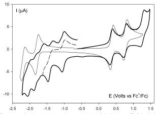
*Figure 3.* Cyclic voltammetry (v = 0.1V/s) of ZnTPP and **Zn3** in PhCN + 0.1 M Bu<sub>4</sub>NPF<sub>6</sub>. Hair line: CV of ZnTPP (8); bold line: CV of **Zn3**; dashed line: CV of **Zn3**, reverting the scan at -1.6 V.
