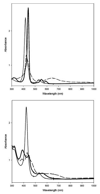
Figure 6. Spectra of the cobalt(II) species (line), the one-electron oxidized species (bold line), and the two one-electron oxidized species (dashed line) obtained during spectroelectrochemical oxidation of 9 (upper) and Co3 (lower) in benzonitrile and 0.1M Bu<sub>4</sub>NPF<sub>6</sub>.
